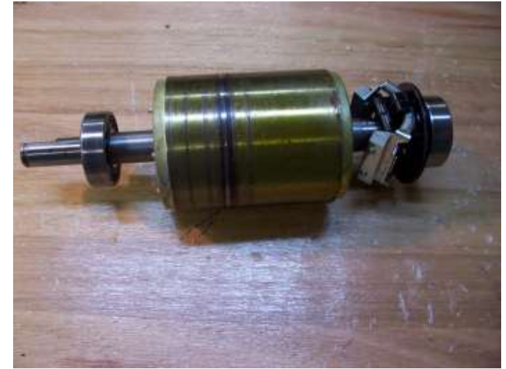
Vacuum pump rotor and centrifugal switch
